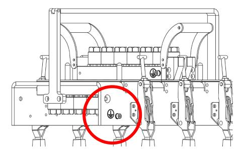
2. Please connect the grounding wire to the marked grounding point on the Color Change Manifold and ensure that it is correctly grounded.
