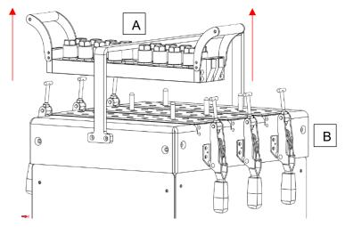
Move the manifold of the color to be cleaned to the purge position and clamp to secure in position.
